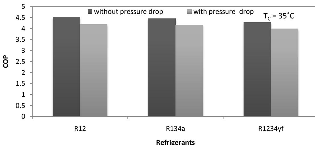
Fig. 3.7 shows variation in COP with and without pressure drop in the evaporator and condenser at  $T_C = 35^\circ\text{C}$ .
